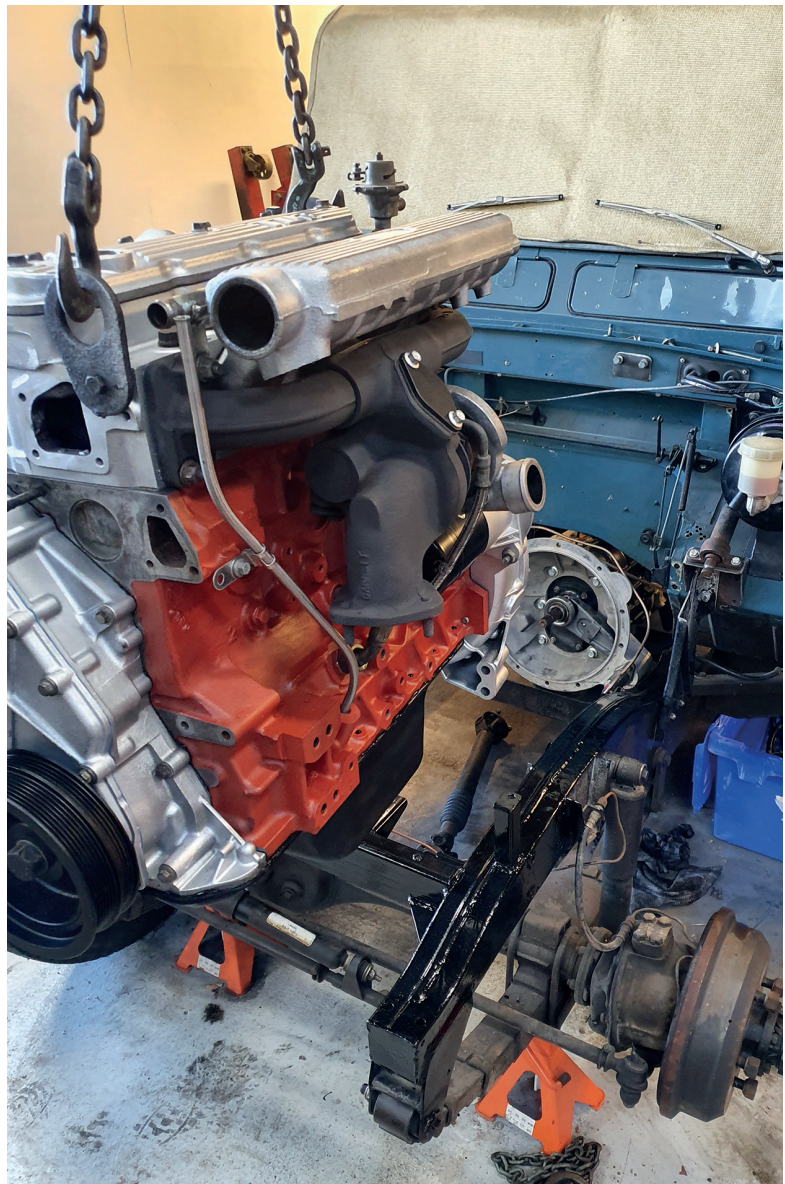
Lowering the new 300Tdi engine into position
