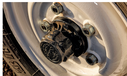
Double-skinned safari roof (left) and freewheeling front hubs (right)
