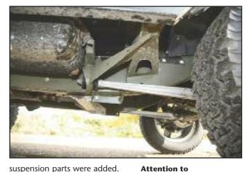
suspension parts were added. Shocks and springs were all new, of course, and Terry opted for Terrafirma items here. These are silver coloured, and match up beautifully with all the other silver-coloured metal work on the underside. Brake discs were replaced with slotted and grooved ventilated discs at the front, while drums were retained at the rear.
