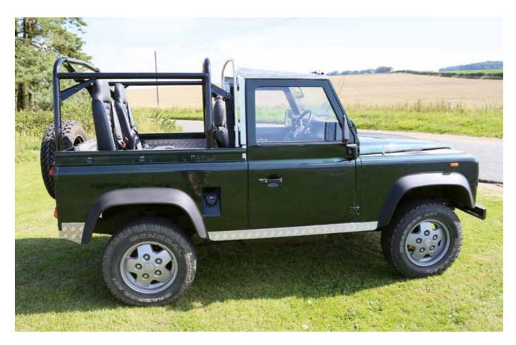
he 200Tdi series Defender was a landmark model when it was introduced in 1990. The new turbodiesel was by far the most potent oil-burner ever to put in an appearance in a Land Rover utility. In fact it was the first designed turbodiesel, because the earlier Turbo Diesel essentially consisted of a turbocharger bolted on to the existing 2.5 naturally-aspirated diesel.
